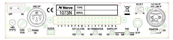
**Power Switch:** This is used to power on/off the unit in stand-alone mode. It has no function when used in a rack or console.
