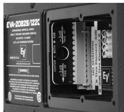
Figure 11c: EVA input panel, with the switch card inserted to shade the upper HF element 3 dB
