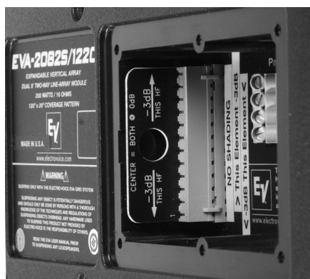
Figure 11a: EVA input panel as supplied, with the high-frequency (HF) shading switch card in its central, 0 dB position
