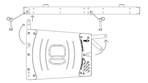
**Step1.** - Pull the joints out, insert them on the frame and lock them with locking pins. Insert two locking pins on the front joints, and one on the rear joints. To obtain a  $0^{\circ}$  alignment between the frame and the LA122, you need to lock the rear joints on the upper hole. **Verify that the locking pins are locked.** See below:
