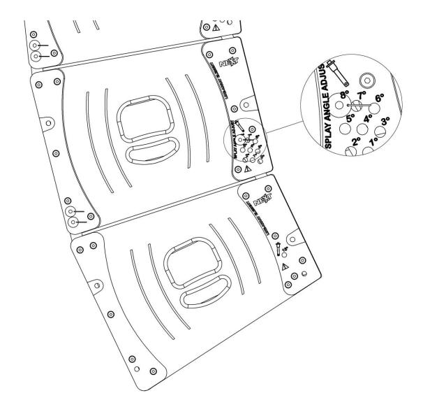
Step 3 - Insert the LA122W on the system in the 8° position. Verify that the locking pin is locked.
