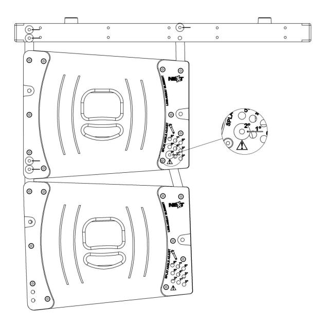
Step 2 - Repeat step 1, this time inserting the LA122 in the previous one. As you can see on the image, the locking pin is inserted in the 2° angle. Repeat the process for the next two LA122 elements for angles 4° and 8°. Always verify that the locking pins are locked.
