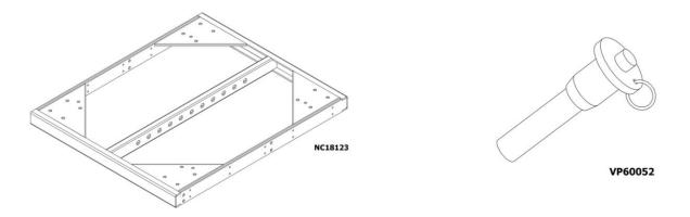
Never use any lock pins but the ones supplied by NEXT-proaudio. These pins are built to withstand the system's weight with a good safety factor. They are also built with very specific dimensions. Also, before you suspend the system, please read the instructions in the "Safety First" chapter.
