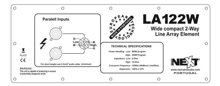
The 4 pins of the two Neutrik® NL4 SpeakON® sockets are wired in parallel within the enclosure. Either connector can be used to connect to the amplifier or another LA122/LA122W element. Please notice that LA122/LA122W Line Array elements are bi-amp only. They were not designed to work in full-range. See the table and the diagram below:
