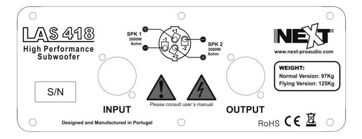
The 4 pins of the three NL4 SpeakON® sockets are wired in parallel within the enclosure. Either connector can be used to connect to the amplifier or another subwoofer. Please notice that each speaker is connected independently for greater versatility and better power handling. See the table and the diagram below:
