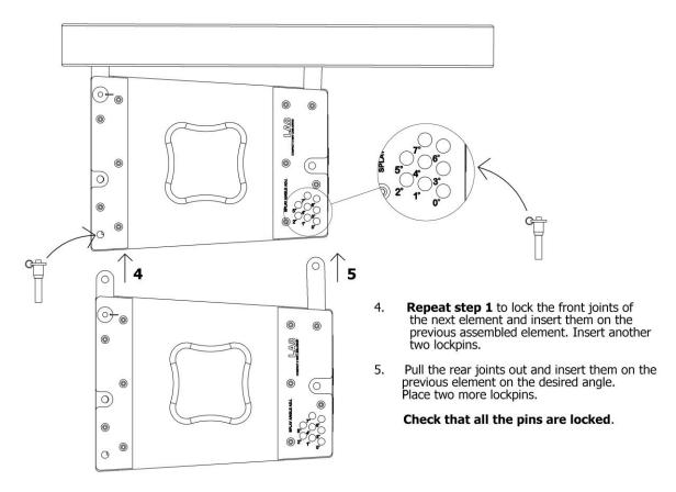
Here's an example of a four element system with 2°, 5° and 7° angles:
