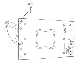
Pull the front joints out and insert a lockpin on the alignement hole. This lockpin will hold the joint in place and prevent the system from articulating while in the air. Check if the pin is locked on.
