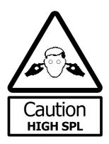
LA8v2 line-array systems are capable of producing extremely high sound pressure levels and should be used with care. Hearing loss is cumulative and can result from levels above 90dB if people are exposed for a long period. Never stand close to loudspeakers driven at high levels.
