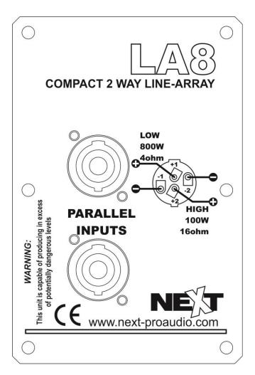
The 4 pins of the 2 Neutrik® NL4 Speakon® sockets are wired in parallel within the enclosure. Either connector can be used to connect to the amplifier or another LA8v2 element. Please notice that LA8v2 line-array element is bi-amp only. Despite having a crossover network it wasn't designed to work in full-range. See the table and the diagram below:
