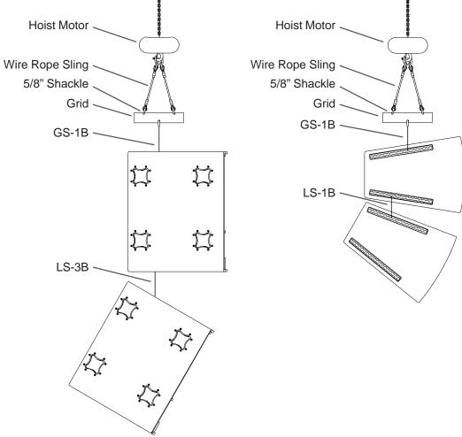
**Figure 2.1a:** *Rigging Hardware on the Top and Bottom of the Enclosures* ELECTRO-VOICE® XI-A Rigging Manual
