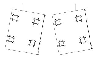
Figure 2.5a: Enclosure Oriented so the Rigging is on the Top or Bottom
