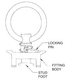
Figure 2.4b: RS-2B Single-Stud Fitting
