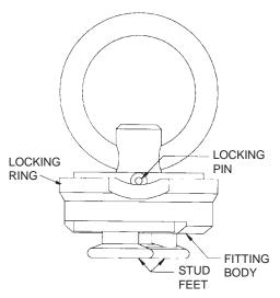
Figure 2.4a: RS-1B Double-Stud Fitting
