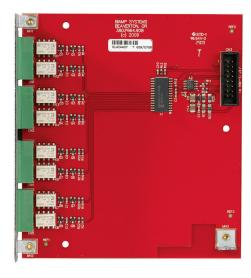
The PARM-1 Page Active Relay Module is an optional module for the VA-8600 and VA-8600c amplifiers. It provides an SPDT relay contact connection for each VA-8600/VA-8600c amplifier channel (total of 8 relays). A relay will be energized when paging is active in the corresponding AM-600 amplifier channel.
