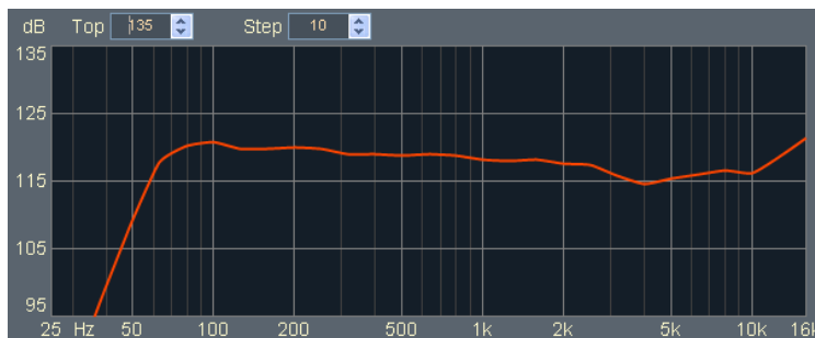
Figure 14 – 6 GTO, simulated on-axis response
