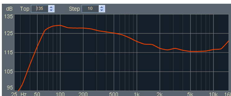
Figure 16 – 15 GTO, simulated on-axis response
