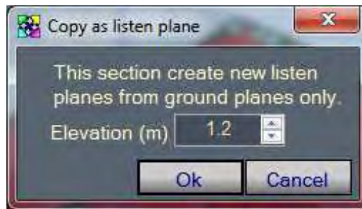
Figure 27 - Panel for creating a “Listening” plane starting from an existing « Ground » plane
