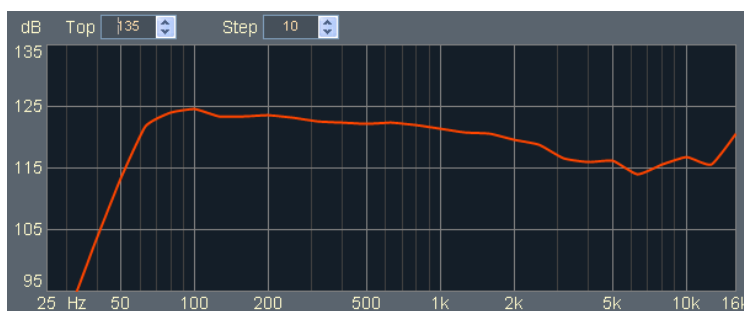
Figure 15 – 9 GTO, simulated on-axis response
