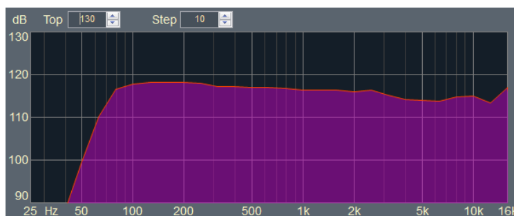
Figure 15 – 9 GTO C-12, simulated on-axis response
