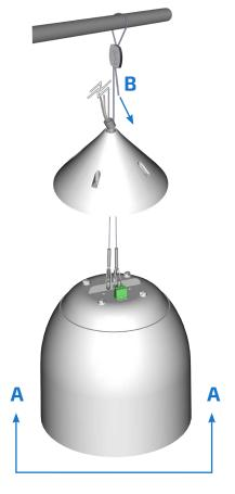
Figure 6. Adjust height of the loudspeaker
