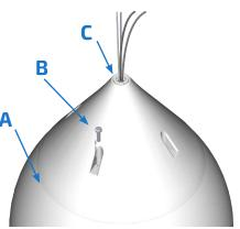
**Figure 8.** Extra silicone adds more weather resistance (A,C); secure cover (B)
