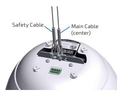
Figure 1. Support and safety cable placement
