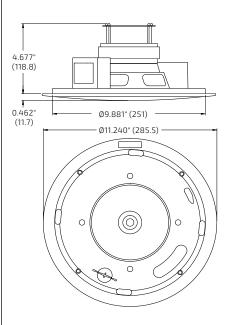
Figure 23. D6 Loudspeaker dimensions
