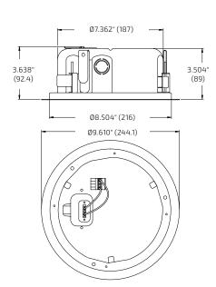
Figure 19. D4LP Back can dimensions
