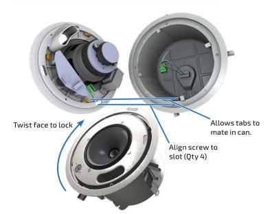
Figure 14. Four Twist-Assist<sup>TM</sup> face tabs inside the back can instantly secure the loudspeaker to the back can with a twist.
