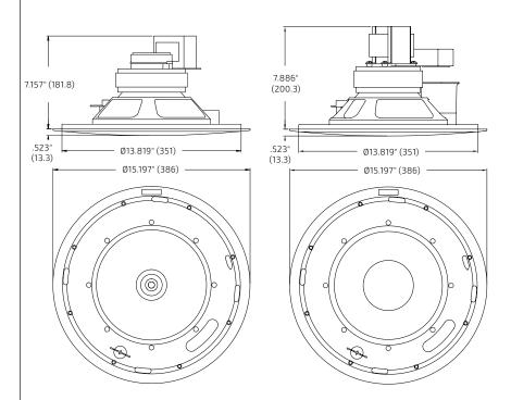
**Figure 27.** D10 (left) and D10SUB (right) Loudspeaker dimensions **Note:** The D10SUB loudspeaker uses the same D10 back can as the D10 loudspeaker.
