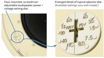
Figure 17. Setting Loudspeaker Tap
