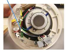
Close-up view of socket for the wiring connector from the back can.
