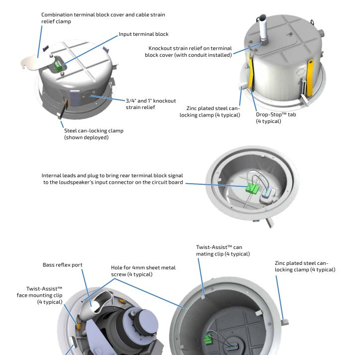
**Figure 1.** Component part identification (1 of 2)
