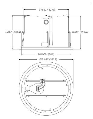
Figure 24. D8 Back can dimensions
