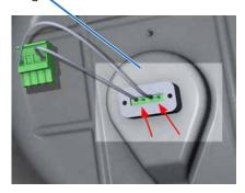
View of 6.5" loudspeaker showing the location of the socket for the wiring connector from the back can.
