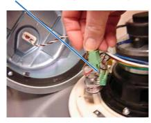
The loudspeaker is now connected to the wires from the can and is ready to mount in the can.
