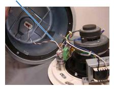
Figure 4. Internal wiring between can terminal block and loudspeaker
