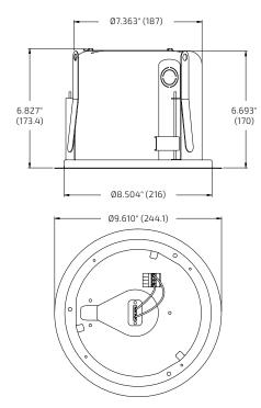
Figure 18. D4, D5, D45 Back can dimensions
