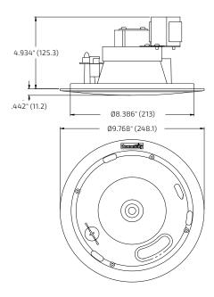
Figure 21. D5 Loudspeaker dimensions
