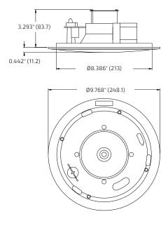
Figure 20. D4 Loudspeaker dimensions
