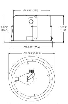
Figure 22. D6 Back can dimensions
