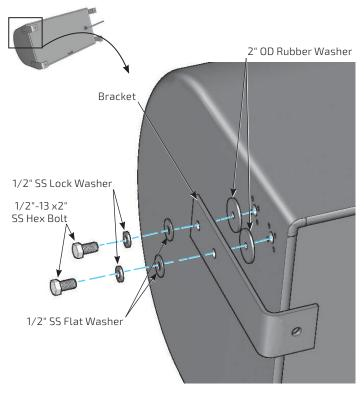
Figure 6. Bracket attachment to subwoofer
