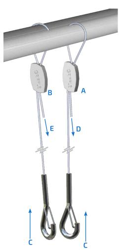
**Figure 3.** Hang the loudspeaker using Gripples
