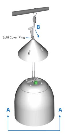
**Figure 6.** Adjust height of the loudspeaker
