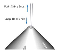
**Figure 2.** Thread cables through the loudspeaker cover
