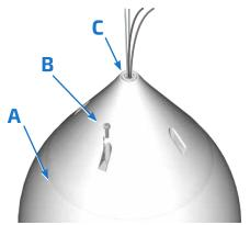
**Figure 8.** Extra silicone adds more weather resistance (A,C); secure cover (B)
