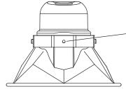
Single 13mmØ fixing point; suitable for 12mm or 1/2" bolts.
