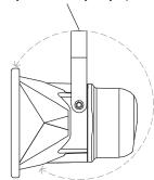
Single 13mmØ fixing point; suitable for 12mm or 1/2" bolts.
