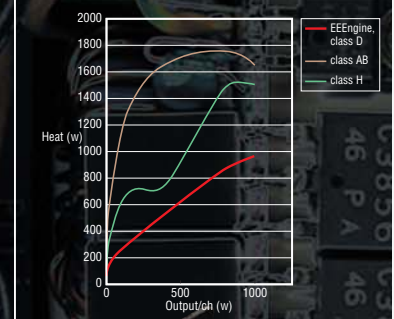
Figure 4: Efficiency comparison data (heat generation level vs. output)
